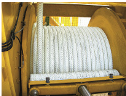
Wire rope after 6 months and 37 immersions between 150m and 500m
