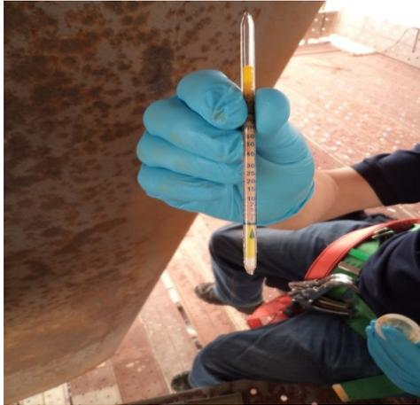
Substrate tested for Chloride content
