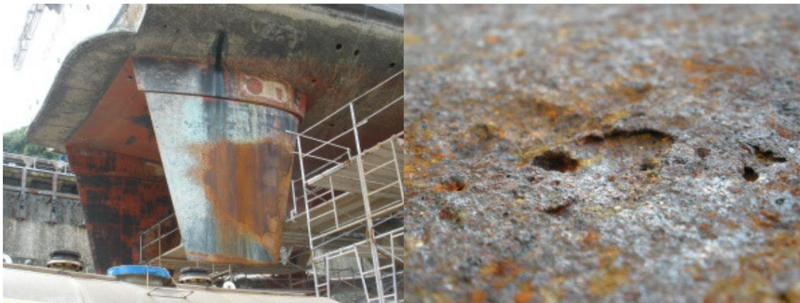
Metal pitting caused by cavitation and corrosion
