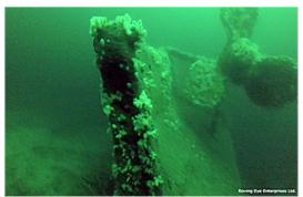
Stern of the vessel showing the portside bronze propeller.
