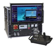
The new surface control consul incorporates Saab Seaeye's iCON behaviour-based intelligent control software.
